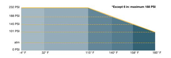
The maximum working pressure of the Transair® system versus the operating temperature can be seen in the diagram below.
